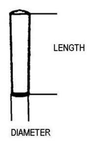
When measuring Metric Tapered pins, the diameter is measured at the smallest end of the pin.
